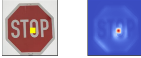
Figure 6.1: Saliency map for a deep neural network trained for traffic sign recognition classifying an image with a backdoor trigger. Red color in the saliency map indicates high importance whereas blue color indicates irrelevance.
